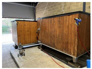
Two Timber clad jacketed, elevated open top fermentation vessels, approx 1650 x 2600mm, with Danfoss digital temperature display Stainless steel jacketed vertical liquid storage vessel, c. 2000 litres, with heating element (CIP)
