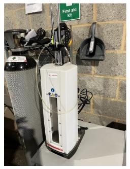
Anton Pevar PFD filling device with control unit
